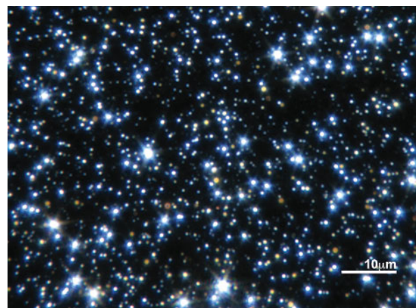
Figure 2. Wet mount of copper particles viewed via enhanced dark field microscopy. This figure highlights the non-quenching resonant light scattering characteristic of the metal NP used in this study. Wet mounts of NP resembled a deep field of stars, with the different intensities and colors of light likely reflecting the sizes of the NP or NP aggregates responsible for each signal.
